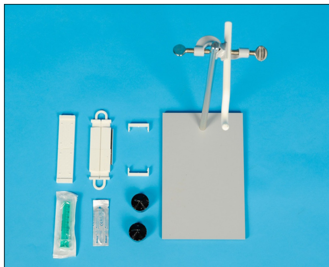
Figure 1. Experimental setup for bedside tensile elongation measurement, including the hanging device, securing clamps, stand, and standardized 400 g load.
