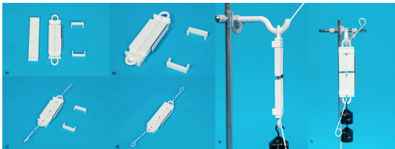
Figure 2. Elasticity assessment step by step: a) connecting element, hanging device and two clamps; b) hanging device placed on connecting element; c) stent placed on hanging device; d) stent secured by two clamps; e) connecting element removed and 400 g weight attached to hanging device; f) final configuration with 400 g weight attached.
