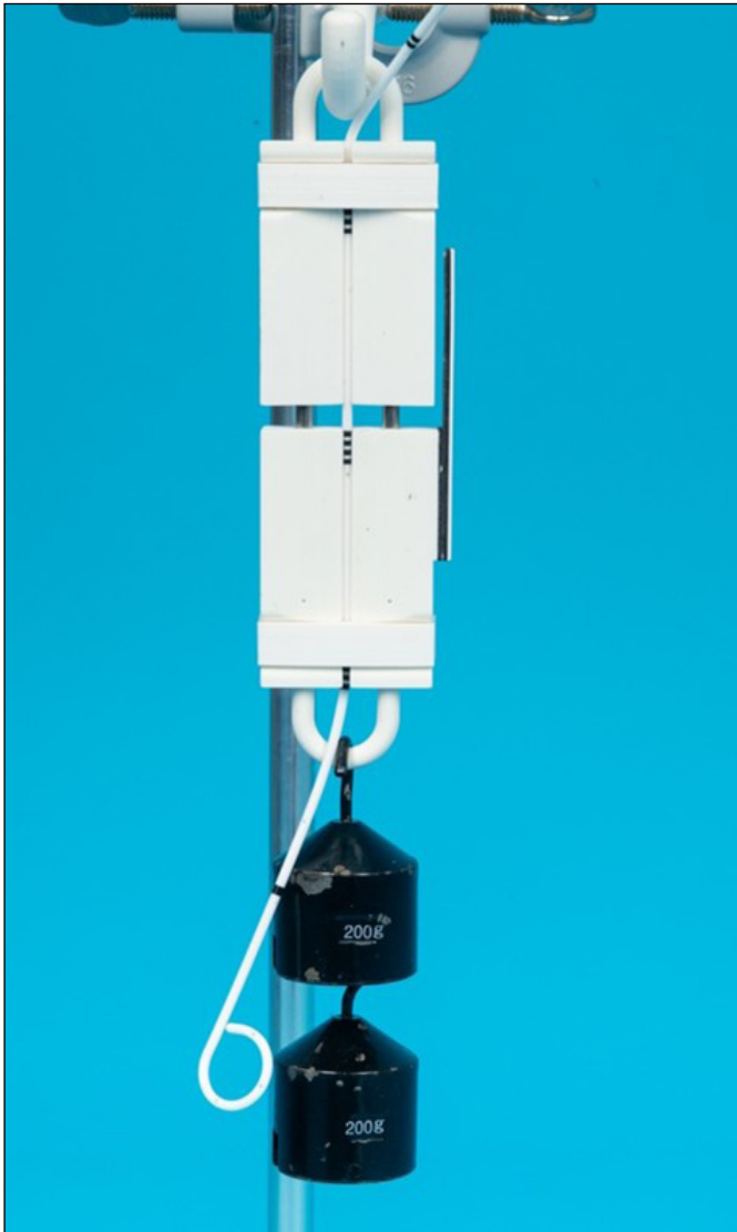
Figure 3. Hanging device with removed connecting element and secured stent with 400 g weight attached.
