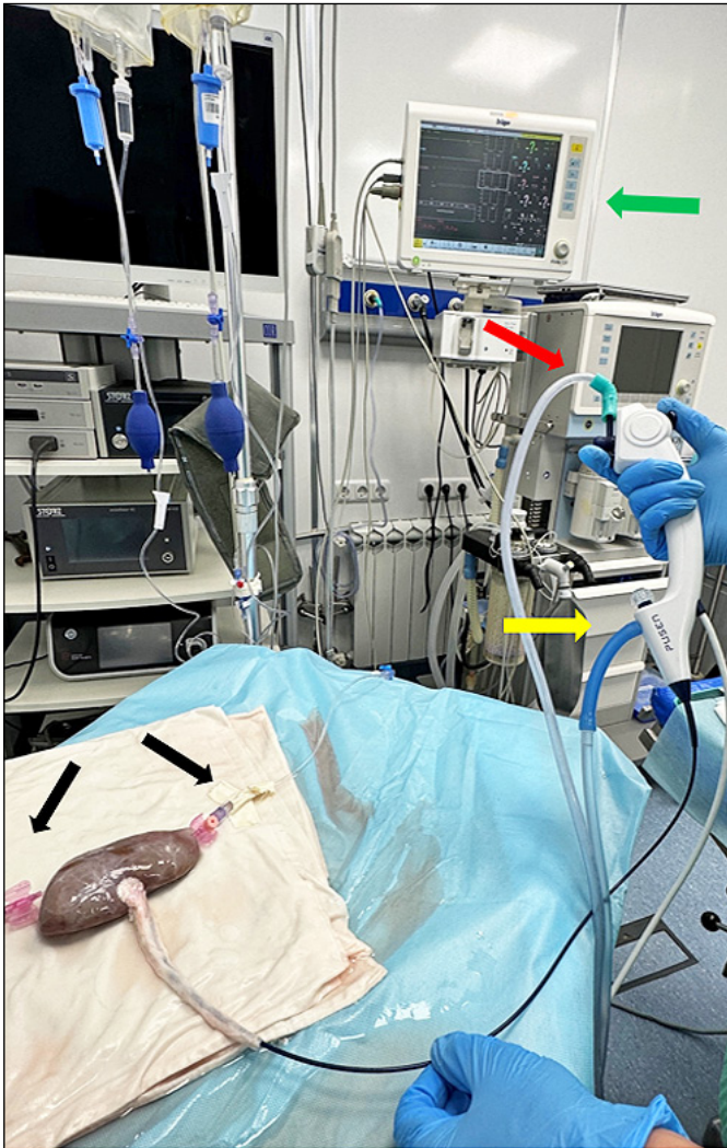
Figure 1. Experimental setup. Black arrows – arterial catheterization system connected to 18 Gauge intravenous catheters placed in the lower and upper calyx; yellow arrow – irrigation system connected to the irrigation canula; red arrow – aspiration canula; green arrow – pressure monitor.
