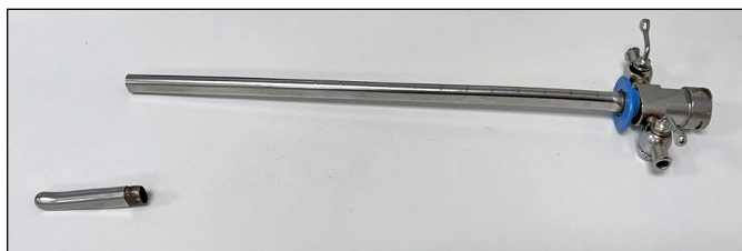
Figure 3. Cystoscope sheath and the detached distal metallic tip.
