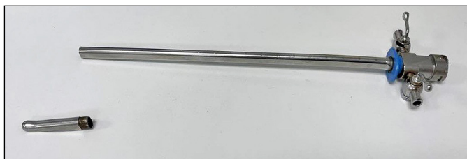
Figure 3. Cystoscope sheath and the detached distal metallic tip.
