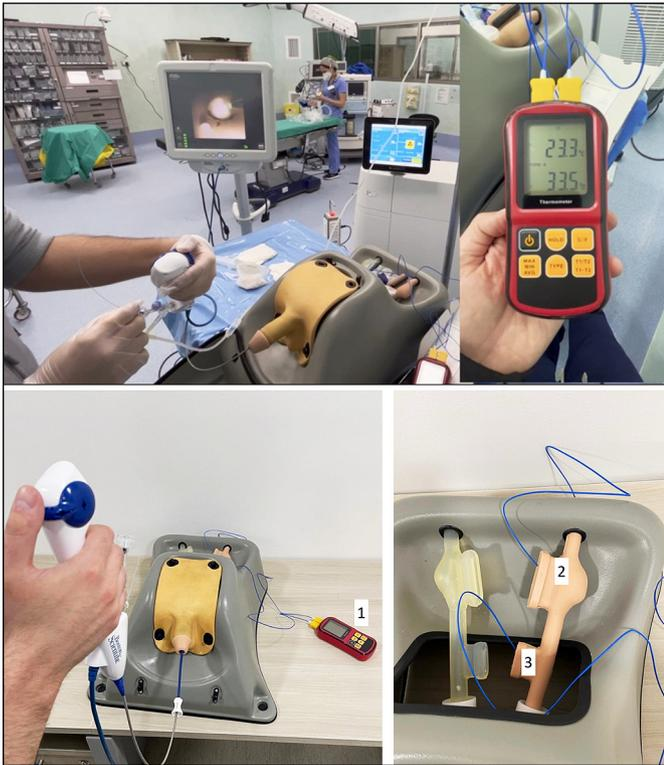
**Figure 1.** Experimental Setup: (1) Thermometer (2) Thermocouple at renal pelvis (3) Thermocouple at proximal ureter.
