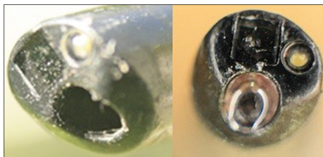
Figure 7. LithoVue before and after use.
